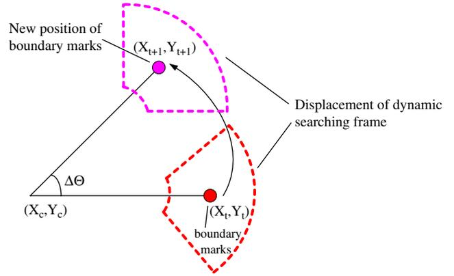
Fig. 5. Displacement of dynamic searching frame.
