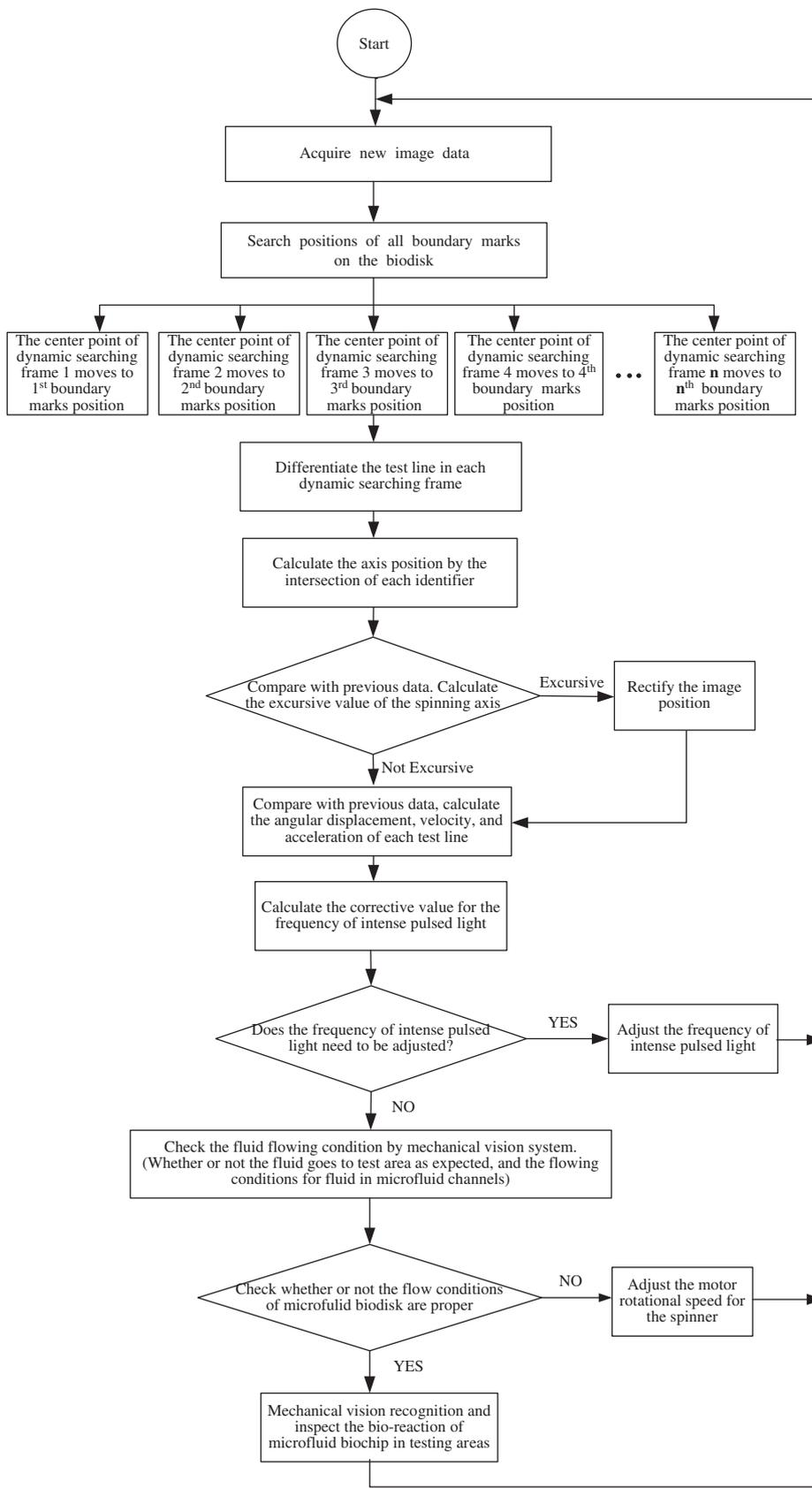
Fig. 6. Flow chart for the algorithm of mechanical vision system in the biodisk.
