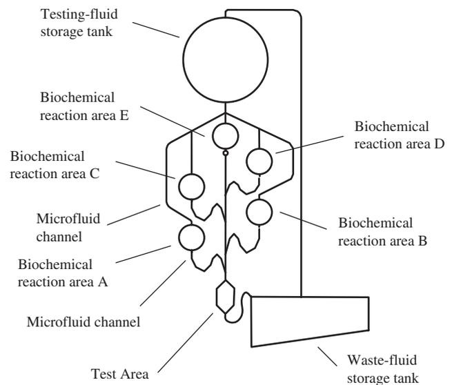
Fig. 3. Structure of testing zones in the microfluidic biodisk.
