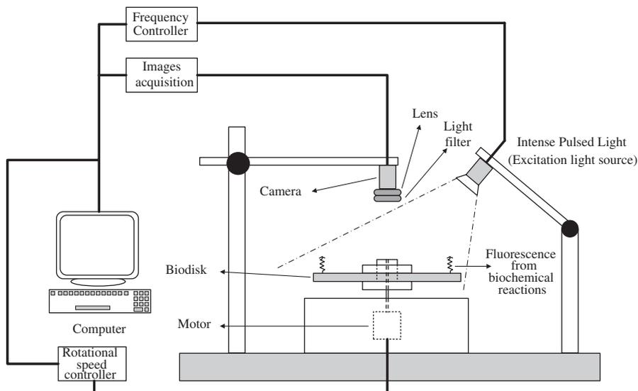
Fig. 9. Structure for the light field inspection system of the biodisk and the spinner.
