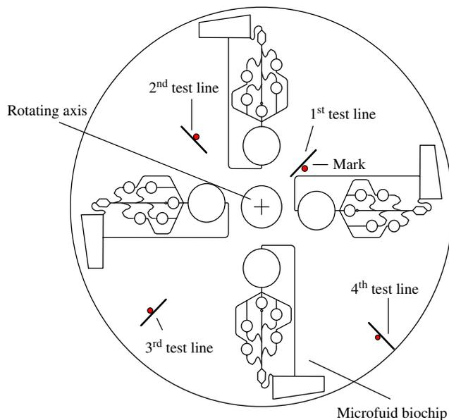
Fig. 2. Layout of the microfluidic biodisk.
