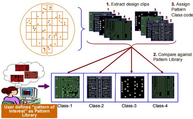
Figure 3. DBC: Supervised binning methodology help detect known systematic excursion
