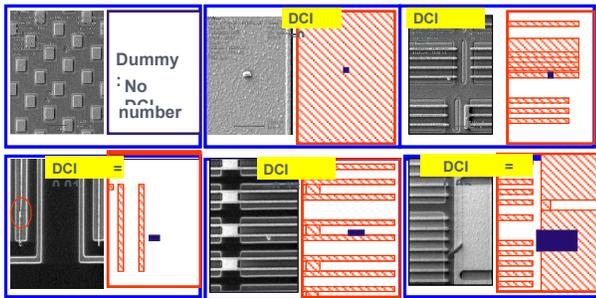
Figure 8. DCI samples shown defect size and pattern background information
