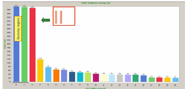
Figure 6. DBB: un-Supervised binning results on wafer #4. Top Pareto bin is defect on dummy pattern
