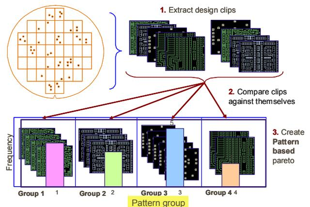
Figure 2. Design based binning method: taking design and inspection information to identify potential systematic pattern problem
