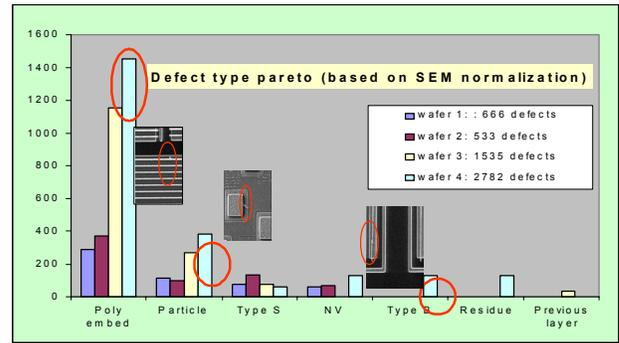
Figure 5. Traditional method for review sampling and normalization
