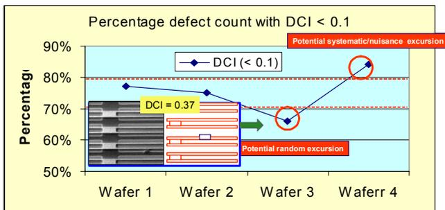
Figure 9. DCI chart shown wafer # 3 had potential random excursion as in SEM picture
