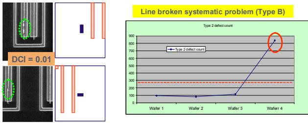
Figure 7. DBC binning results shown wafer #4 had systematic excursion as in the SEM pictures
