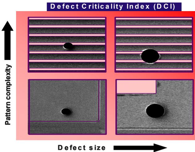
Figure 4. DCI: Random defect management using Design and defect size information
