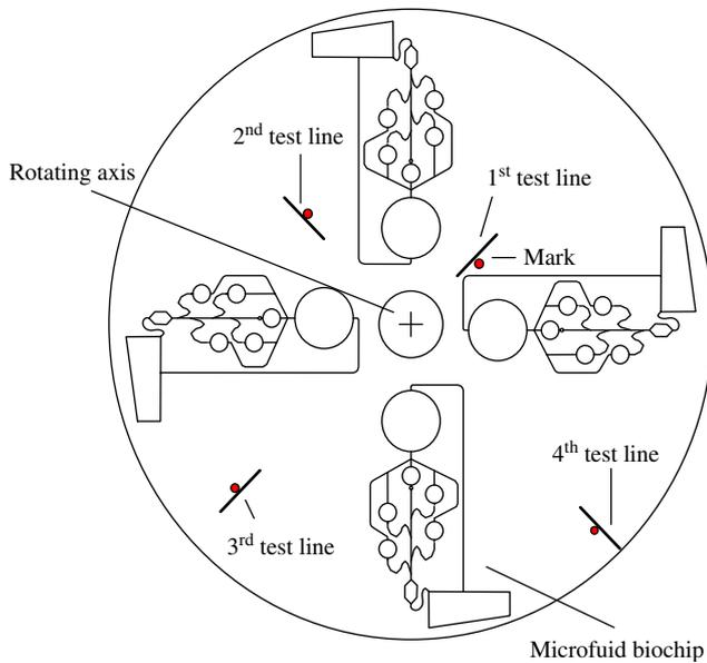
Fig. 2. Layout of the microfluidic biodisk.
