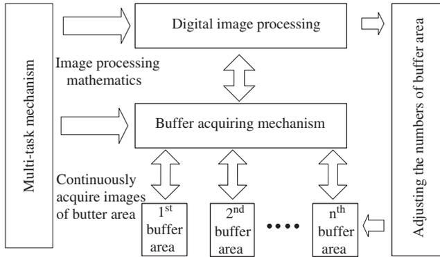
Fig. 7. Diagram for the rules of rapid image processing and adjustment of memory spaces.
