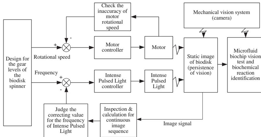
Fig. 10. Flow chart for the light field inspection of the biodisk and the spinner control.
