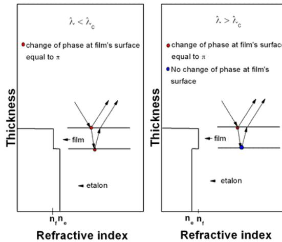
Fig. 6 A wavelength dependence of the change of phase on reflection of light at the surface film - etalon
