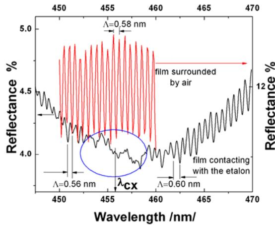
Fig 9 Reflectance in direction of fast axes from film contacting with the etalon and from film surrounded by air; the measured value of the quasi-period at different wavelength is shown
