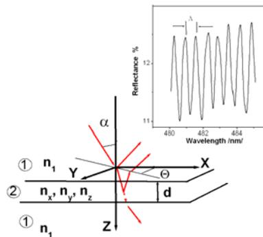
Fig. 1 The film under the measurement and typical denotes used; the spectral response of reflected light represents a channel spectrum with a period  $\Lambda(\lambda)$ .
