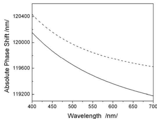
Fig. 4 Different results for the absolute phase shift determined from measured channel spectra; dashed curve – random deviation from “true” peak positions  $\pm 0.2nm$  ; solid curve – deviation lower than  $0.05 nm$
