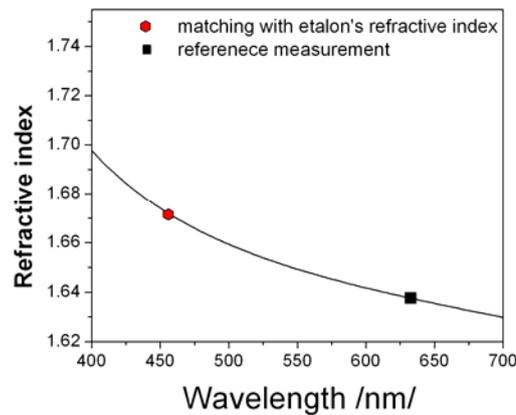
Fig. 10 The refractive index of fast axes determined according to Eq. 3;  $n(\lambda_c)$  and  $d$  found from modified channel spectrum (Fig. 7b) and Eq.4
