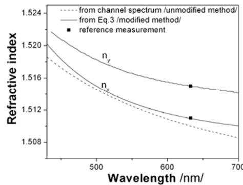
Fig. 11 A comparison between the results of unmodified and modified method; the modified method provides higher accuracy data
