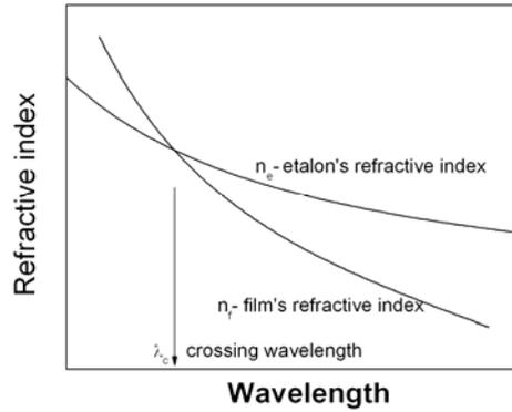
Fig. 5 Dispersion curves of the etalon and of the film; at the crossing wavelength  $n_e = n_f$
