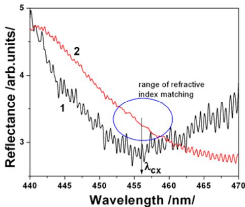
Fig. 8 An experimental confirmation of the based idea of the method of measurement; 1 - the spectrum of reflected light in direction of slow axes; 2- the spectrum of reflected light in direction of fast axes; the range of equal crossing of refractive indices is marked.
