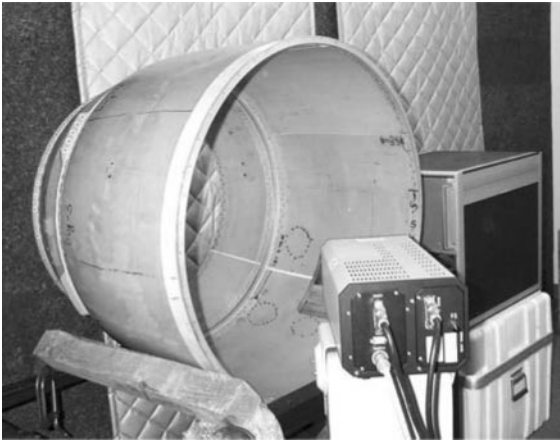
2 Jet engine casing undergoing testing: scanning LDV is in foreground and the shockwave generator behind casing
